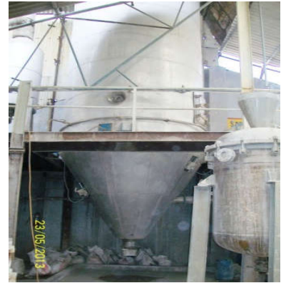
Spray Drier Capacity - 500 Kg/Hour
