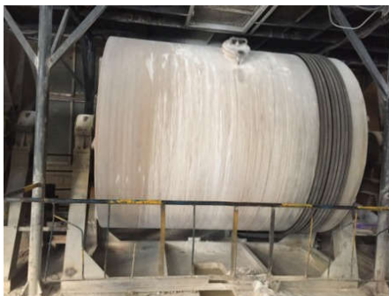
Ball Mill Capacity 3 MT/ Batch
