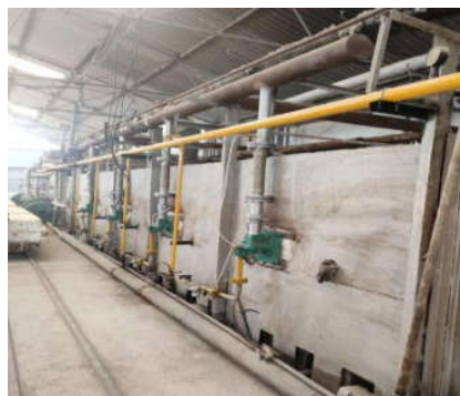
Shuttle Furnace suitable for 1520°C - Capacity - 1.5 MT/Batch
