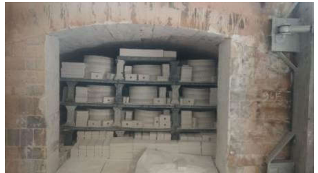
Shuttle Furnace suitable for 1520°C - Capacity - 1.5 MT/Batch
