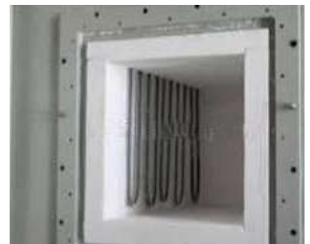
Shuttle Furnace suitable for 1520°C - Capacity - 1.5 MT/Batch
